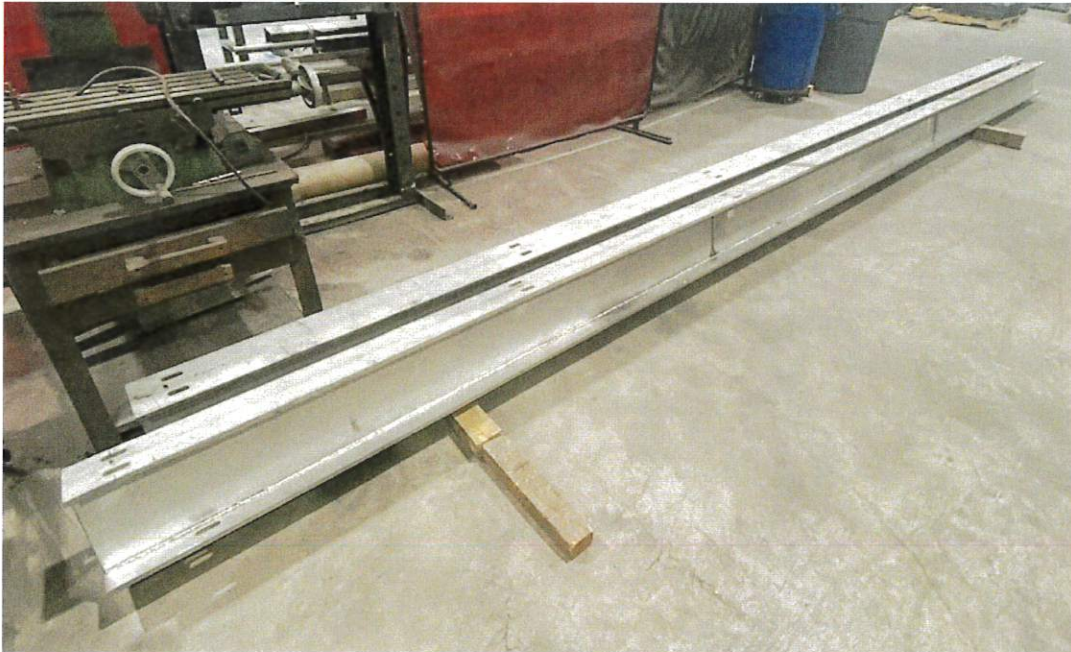
Production of Sludge Collection Trough Supports were near completion. All materials for the proposed S.S. Sludge Collection Troughs have been acquired.
