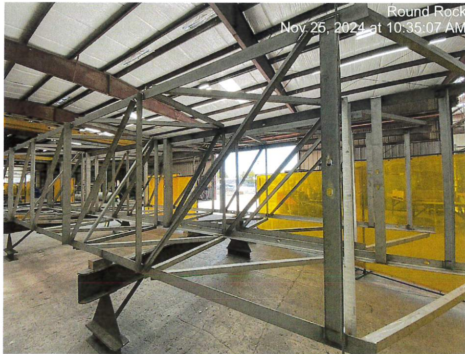
Production of Two (2) S.S. Collector Rake Arms was near completion during inspection.
