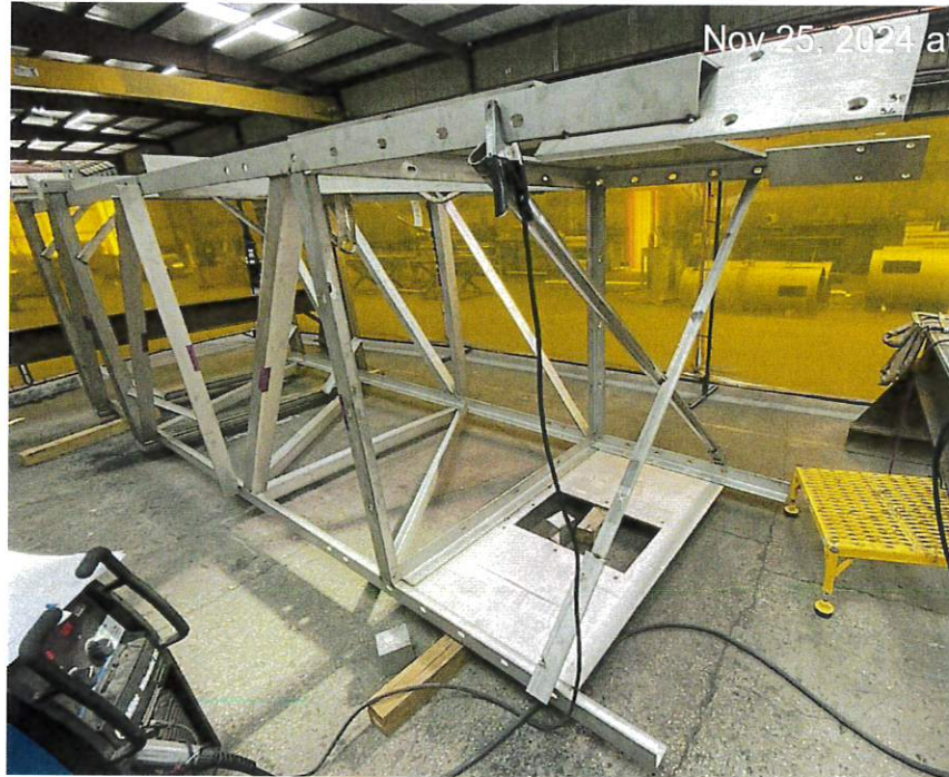
Production of 5' Square S.S. Drive Cage was near completion during inspection.
